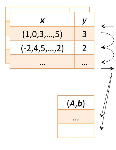
Aggregation phase 1 on each node: 1. Initialize: (A, b) = (0, 0)Transition for all rows: 2.  $(A, \mathbf{b}) = (A, \mathbf{b}) + (\underbrace{\mathbf{x} \cdot \mathbf{x}^{\mathsf{T}}, \mathbf{x} \cdot \mathbf{y}}_{\text{map}})$ 3. Send  $(A, \mathbf{b})$  map reduce Aggregation phase 2 on master node: 1. Merge:  $(\overline{A}, \overline{b}) = (\overline{A}, \overline{b}) + (A, b)$
